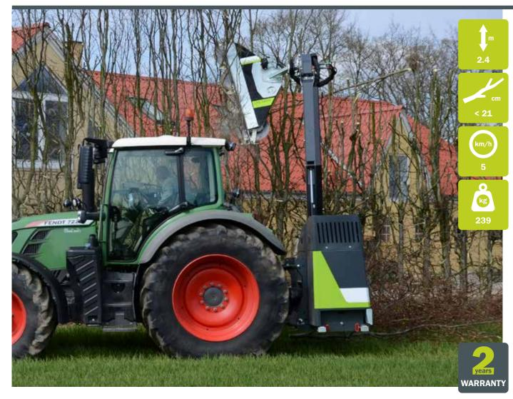
The Quadsaw LRS 2402 is the second largest saw in the series and has an enormous power and capacity. Branches up to 21 cm are cleanly cut - experienced drivers can manage branches up to 40 cm.
