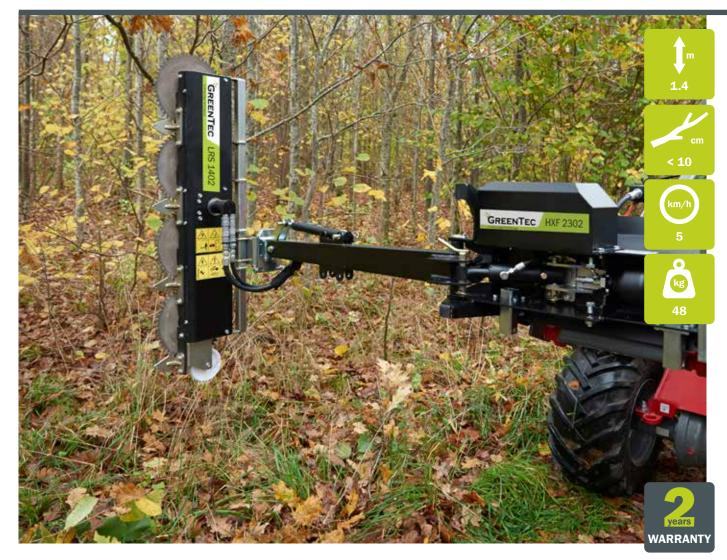
The Quadsaw LRS 1402 is a small yet powerful quadsaw with four saw blades and a working width of 1.4 m.
